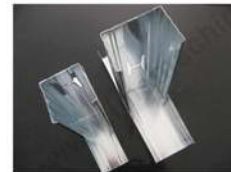
Profile Width Adjustment by Spacers on Rolls
