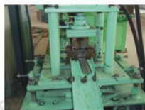
Fire Damper Roll Forming Production Line with Corner Punching
