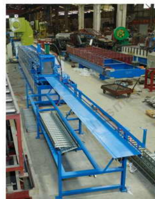
Unistrut Channel C21/41X41X2.5 Roll Forming
